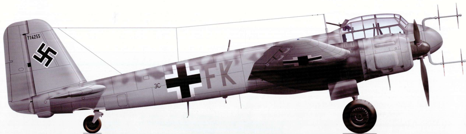
LEFT AND ABOVE: Two views of a Ju 88 G-1 of 2./NJG 4 in January 1945. From August 1944, the parent I. Gruppe, to which the 2. Staffel belonged, was subordinate to Jafü Mittelrhein, but in January 1945 was controlled by the 2. Jagddivision. Note the crew entry hatch offset to starboard and the heavy exhaust staining on the rear of the engine nacelles.
