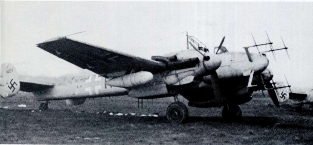
LEFT: This Bf 110 G, G9+AT, had 76 mottling clearly applied over 75 on all upper surfaces, while G9+HT, W.Nr. 160128, was finished in 76 overall with a mottle of 75 over the upper surfaces.
