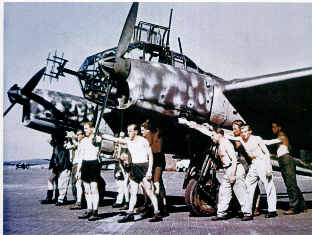
ABOVE: One of the more unusual types provisionally employed in the night fighter role by NJG 100 on the Eastern Front was this Fw 189A. This machine was fitted with FuG 212 radar and a single, obliquely-mounted MG 151 in the rear of the cockpit and which may be seen protruding from the canopy. Up to six Fw 189s were employed by I./NJG 100 between March and December 1944, while II. Gruppe had a similar number but only used them up to October. Although the operational code cannot be seen on the aircraft shown here, known codes are W7+CB, +DB, +EB, +MB, +NL and W7+WM, most of these being Fw 189A-4s with a 20 mm MG FF cannon in each wing root in addition to the oblique MG 151. On this aircraft, the standard factory 70/71 uppersurface scheme has been modified with an overspray of 76 mottles.
