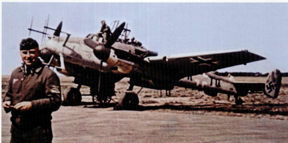
ABOVE: Major Helmut Henz, the Kommandeur of the Truppenversuchskommando – or Service Experimental Attachment – at Werneuchen, seen standing in front of a Bf 110 equipped with SN-2. Note the 74/75/76 camouflage and the yellow areas under each engine cowling which were intended to identify the aircraft as friendly to Axis ground forces and were a widely employed recognition aid.
