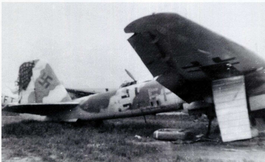
LEFT: Photographed at Fritzlar in Germany in 1945, this Ju 88 G of 6./NJG 2 with the operational code 4R+EP had a most unusual camouflage. Disregarding the dark patch on the tail, which is merely a piece of camouflage netting, the rest of the machine visible in this view has been camouflaged in a disruptive pattern of what is probably 76 and 75. Very few examples of this scheme have been observed, but it is thought that the upper surface of the wings and tailplane were finished in a similar manner.
