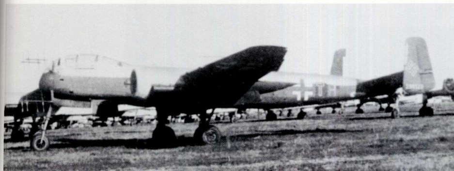
LEFT: This He 219 A-2, W.Nr. 290123, was surrendered at Westerland-Sylt and was camouflaged in the same basic scheme as W.Nr. 290126. This aircraft had flown with I./NJG 1, and although the full operational code was G9+TH, it is not known if the smaller 'G9' was actually applied. Note that on all the aircraft shown on these pages with black undersurfaces, the front engine cowlings were finished completely in 76.
