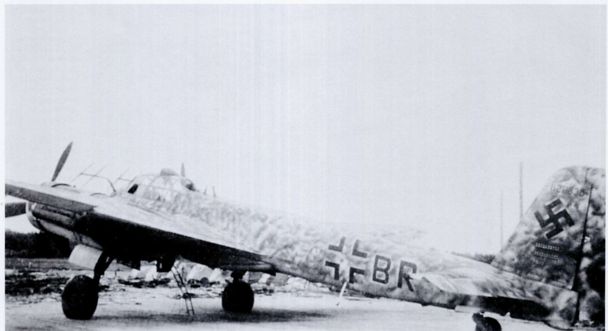
ABOVE: An He 219 A-2 of I/NJG 1 at Münster-Handorf in the winter of 1944/45. Note the black undersurface of the starboard wing, the spiral spinners, and the small Roman VI below the canopy which indicated that this aircraft was equipped with 'Lichtenstein' FuG 220d radar.
