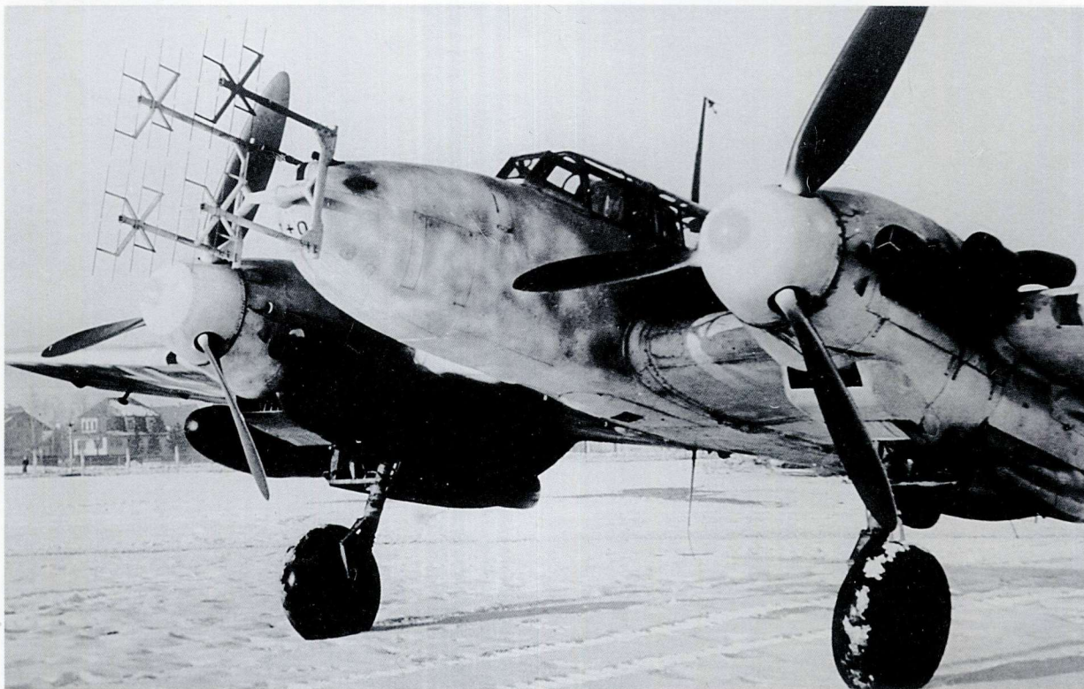
ABOVE AND OPPOSITE PAGE: This Bf 110 G-4 of 6./NJG 6 landed at Dübendorf in Switzerland shortly before midnight on 15 March 1944. The aircraft was fitted with auxiliary fuel tanks and had 76 undersurfaces with most of the starboard wing, including the drop tank, painted black. Note, however, that an area immediately aft of the spinner was not painted black and that the black under the wing terminated in an irregular line just short of the leading edge. The uppersurface colouring is most interesting, for while the nose area approximately forward of the windscreen retained the original factory 74/75/76 finish, the rest of the aircraft's uppersurfaces had been repainted in a low demarcation splinter scheme of 74 and 75. Note that the tactical code 2Z+OP was repeated on the nose and the Werknummer 5547 was applied to the tail.
