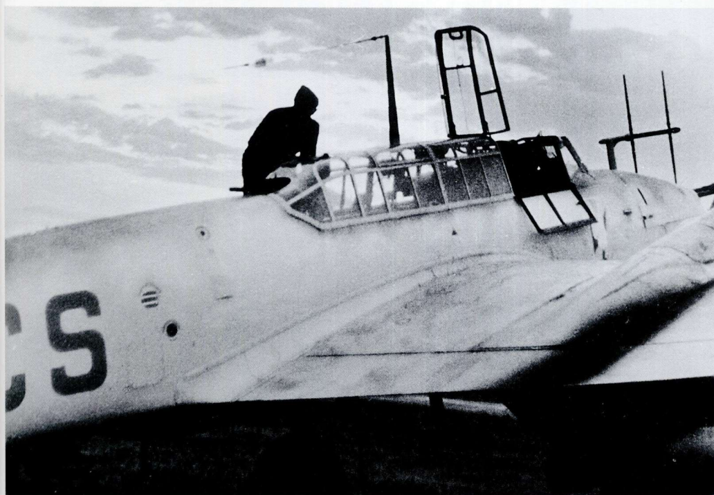
ABOVE: A detailed view of the flame dampers on a Bf 110 G night fighter. Whereas the starboard inner flame dampers directed the exhaust gases under the wing, the other three dampers led over the wings and often resulted in heavy black deposits, as shown on G9+CS of 8./NJG 1 (LEFT).
