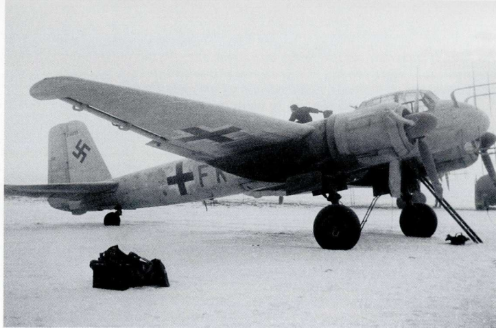
LEFT AND ABOVE: Two views of a Ju 88 G-1 of 2./NJG 4 in January 1945. From August 1944, the parent I. Gruppe, to which the 2. Staffel belonged, was subordinate to Jafü Mittelrhein, but in January 1945 was controlled by the 2. Jagddivision. Note the crew entry hatch offset to starboard and the heavy exhaust staining on the rear of the engine nacelles.
