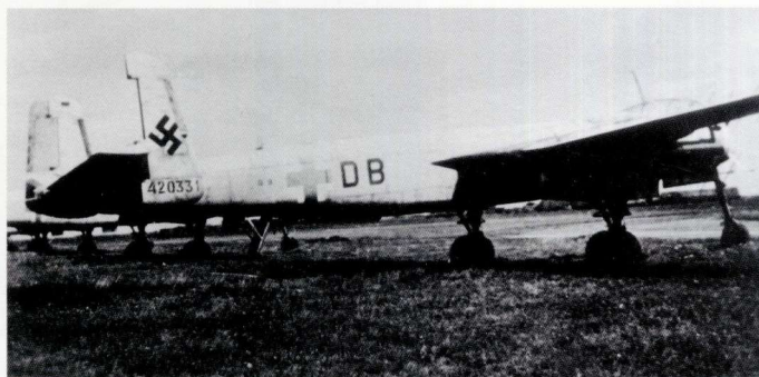
BELOW LEFT AND BELOW: The remains of an He 219 at Halle in 1945. Although the full operational code cannot be recognised, the unit code '1L' of NJGr 10 is just visible in small characters on the fuselage. The two photographs illustrate the third basic type of camouflage applied to the He 219, this example showing that most of the 76 uppersurfaces and fuselage sides have been oversprayed with 81 or 83, or possibly both of these colours. The undersurfaces were 76 but visible in the photograph ( BELOW ) is a hard demarcation line on the engine nacelles between the 76 and what is again probably either 81 or 83.
