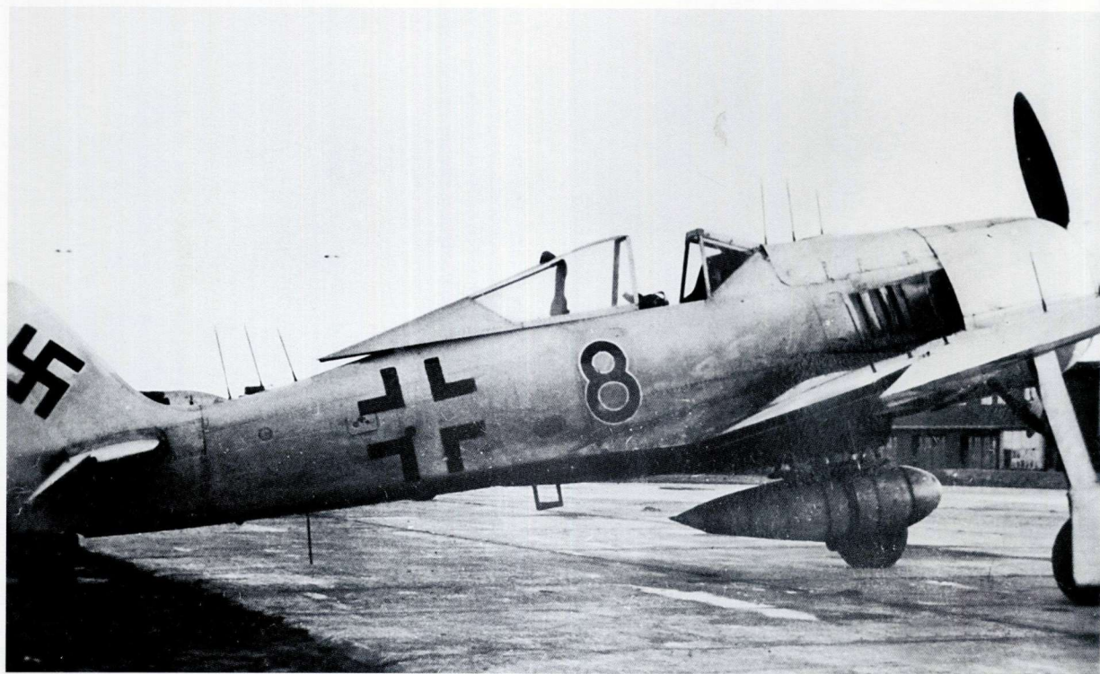
ABOVE: An Fw 190 A-6 coded 'Black 8' of 2./JG 300 in the autumn of 1943 showing the FuG 217 'Neptune' acrials mounted on the wings and in front and behind the canopy.
