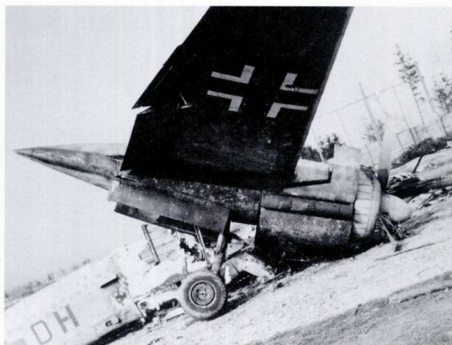
LEFT AND BELOW: This He 219, W.Nr. 290004, was found at Paderborn airfield on 10 April 1945 and was the first example of the type to be examined by the Allies. Although the nose, centre section and left wing were burned out, considerable information was obtained from an examination of the remains. Note that all the tactical code, G9+DH, was in black with the aircraft letter 'D' narrowly outlined in white.
